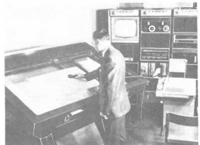
Fig.2. A CADMAC-11 system at Imperial College being used in the input mode.
