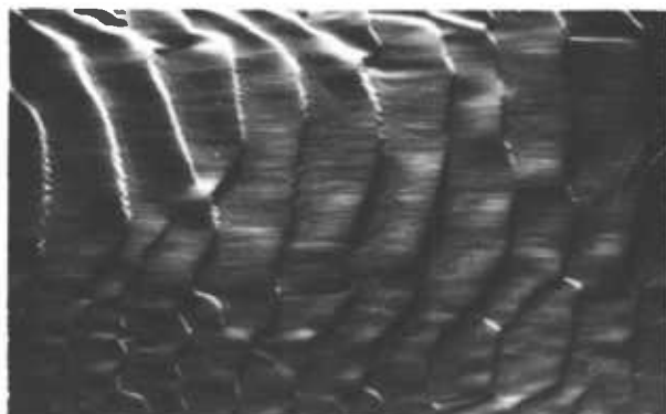
PLATE 5.5. TRANSVERSE PRIMARY RIPPLES FOR THE 15 MICRON GRADE ( \bar{\tau}_0/\bar{\tau}_{oc} = 2.0 )
