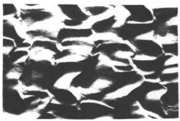
6.6. After 20h. erosion; \bar{\tau}_0 / \bar{\tau}_{0c} = 5.2 (Channel floor exposed in places)
