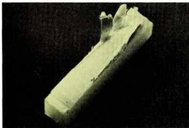
Figure 4. Fracture surface showing the tunneling effect, created by high strength and long crack length combinations. Surface regions yield and slow down cracking.
