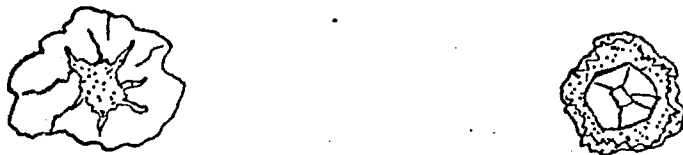
Fig. 5-2(b). Radial-bomb type aggregates with either chalcopyrite (stipple) at the center, or pyrite (white).
