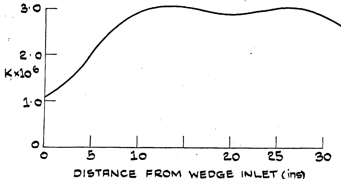
FIG. 3.8: BOUNDARY LAYER IN A PLANE CONVERGENT CHANNEL: VARIATION OF R_2 , H , C_p/2 & K
