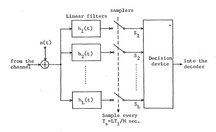
Fig. 1.2(b): Waveform detector
