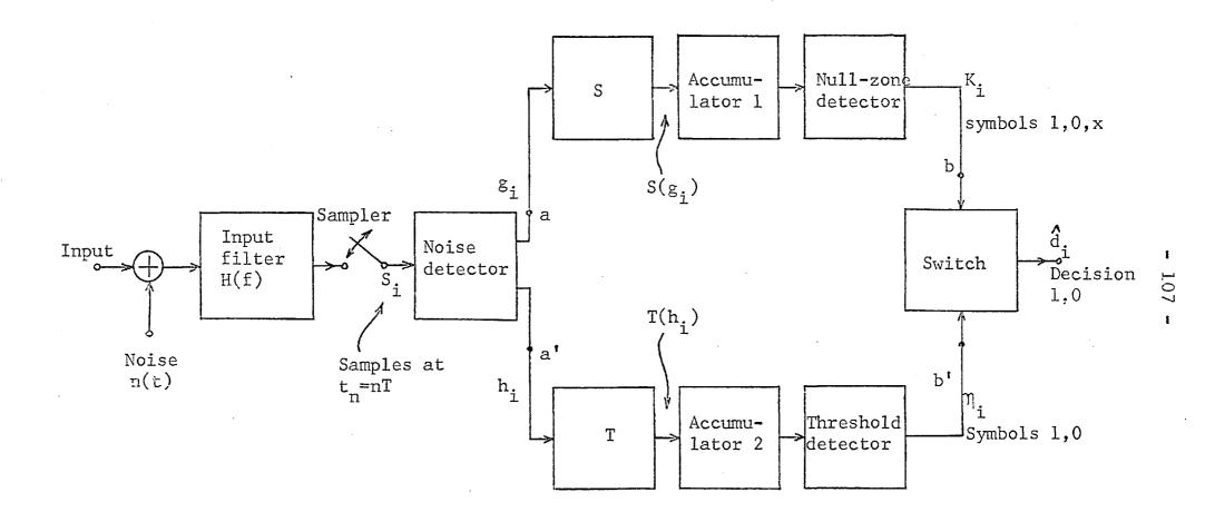
Fig. 5.1: Basic receiver structure.
