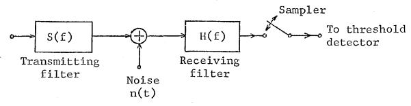
Fig. 4.1: Conventional data transmission system.
