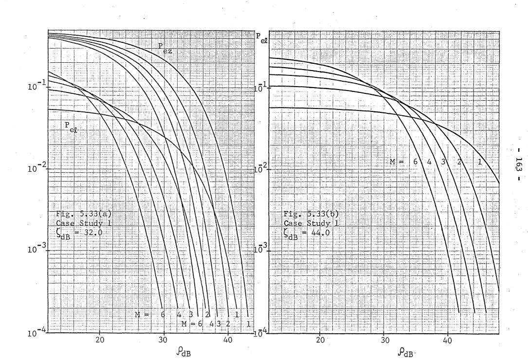
P) Graphs giving the error probability  $P_{ez}$  at the output of the lower branch of the receiver shown in Fig. 5.4, when all samples are corrupted by impulsive noise, that is, when p = 1.
