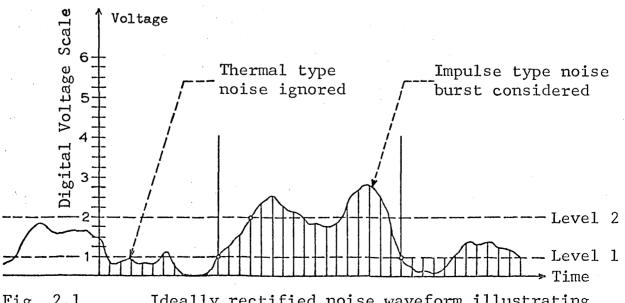
Fig. 2.1 Ideally rectified noise waveform illustrating definition of pulse length.
