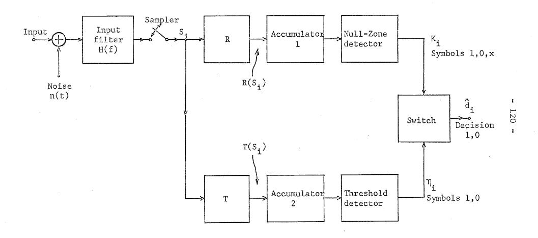
Fig. 5.4: Simplified version of the receiver.
