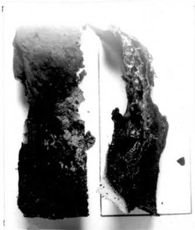
Figure 4.31 ; Sample from ignition experiment after 5 minutes exposure at 25.2 \text{ kW m}^{-2} - Foam A.
