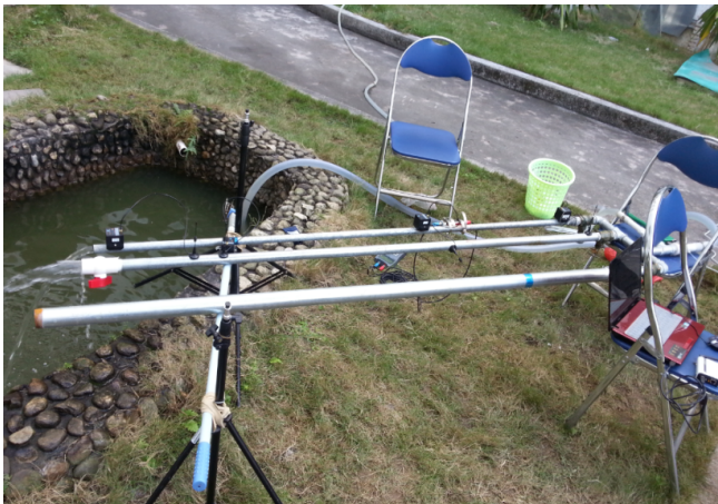
Figure 15. Vibration test experiment of pipelines
