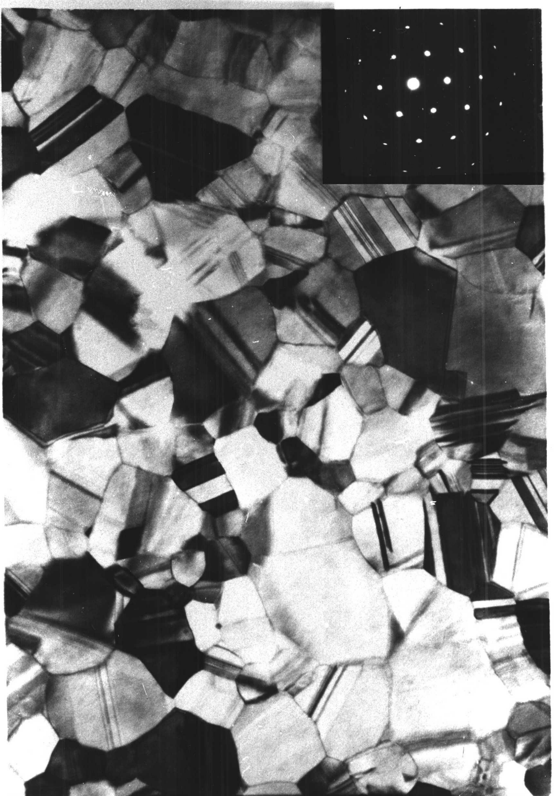
Fig 3.5: Micrograph of a well annealed film ( \times 70\ 000 )
