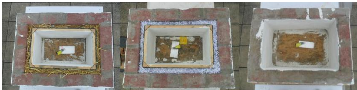
Figure 1. (a) The straw insulation; (b) The shredded paper insulation; (c) Reference model
