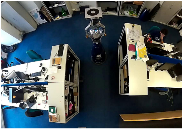
Fig. 5: Example image captured by the ceiling-mounted camera of the external localisation system. The circular marker on top of the robot is used to provide the ground truth for robot self-localization.
