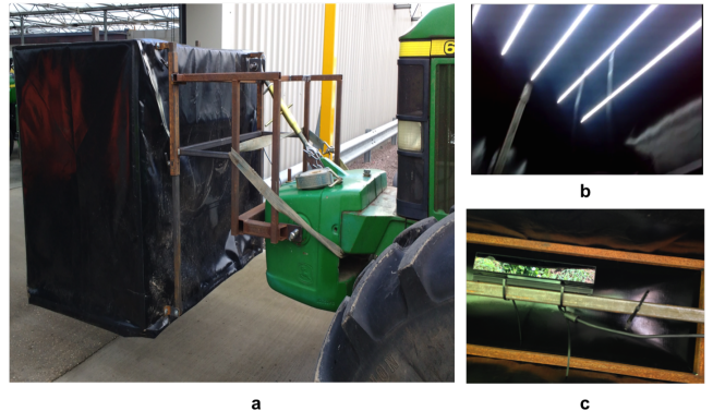
Fig. 2: Enclosure and lighting set-up. (a) Manually adjustable shroud attached to the front of the tractor (b) artificial lighting using LED strip lights (c) inside view of the enclosure with Kinect 2 mounted perpendicular to the field.
