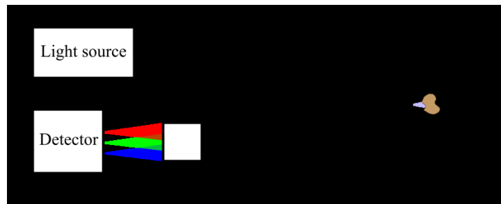
Figure 4.1 Basic configuration of a steady-state fluorescence spectroscopy instrument, utilising a fibre-optic probe for light delivery and collection.
