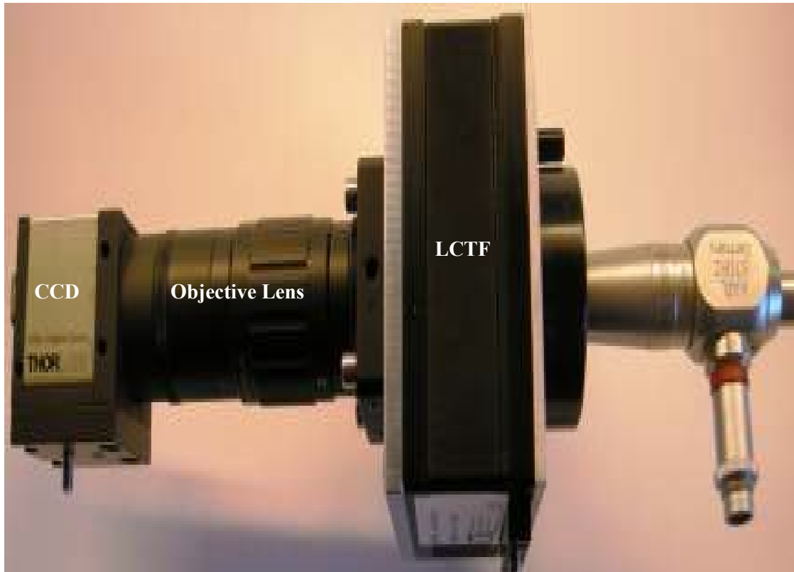
Figure 3.4 Hyperspectral laparoscopic system consisting in a CCD camera and a LCTF attached to a regular rigid laparoscope
