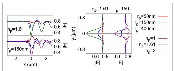
**Figure 8.** |E|-field fluctuations along the *x*-axis (left figure) and *y*-axis (right figure) passing through the centre of the nanoparticle, for polystyrene ( $n_p = 1.61$ ) nanoparticles of  $r_p = 50$  nm (red line),  $r_p = 150$  nm (blue line) and  $r_p = 400$  nm (green line), and nanoparticle of  $r_p = 150$  nm made of  $n_p = 1$  (brown line),  $n_p = 1.61$  (blue line) and  $n_p = 2$  (purple line).
