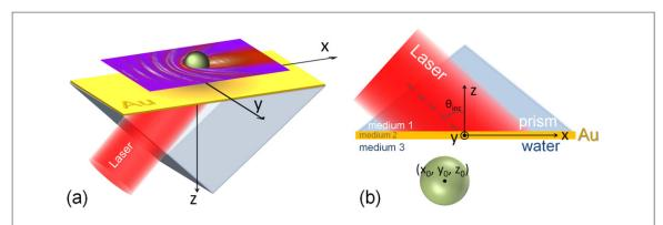
**Figure 1.** The Kretschmann configuration, where a laser is incident on a thin metal film through the prism, exciting a surface plasmon polariton (SPP). (a) An illustration of the SPP diffraction by a nanoparticle. (b) The axes configuration with respect to the Kretschmann set-up. The nanoparticle is positioned with its centre at  $(x_0, y_0, z_0)$ . (figures not in scale)
