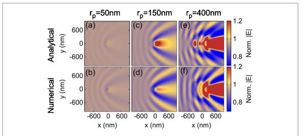
**Figure 4.** SPP diffraction by a polystyrene ( $n_p = 1.61$ ) nanoparticles of various sizes. Top row are analytical predictions and bottom row numerical calculations for nanoparticle radii (a)–(b)  $r_p = 50$  nm, (c)–(d)  $r_p = 150$  nm and (e)–(f)  $r_p = 400$  nm. The plots are normalized to the |*E*|-field when no nanoparticle is present.
