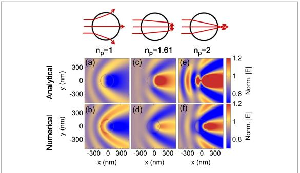
**Figure 5.** SPP diffraction by nanoparticles immersed in water ( $n_w = 1.333$ ) with radius  $r_p = 150$  nm made from different materials (a)–(b)  $n_p = 1$  (i.e. air), (c)–(d)  $n_p = 1.61$  (i.e. polystyrene) and (e)–(f)  $n_p = 2$ . Top figure row illustrates the different ray paths due to the relative change of  $n_p$  with respect to  $n_w$ , middle row are analytical predictions and bottom row numerical calculations for |E| -fields.
