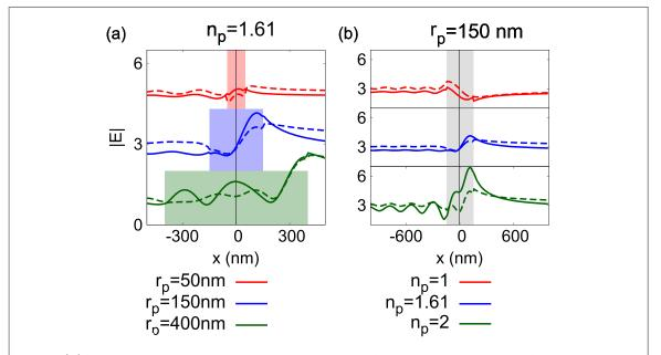
**Figure 6.** |E|-field along the *x*-axis passing through the centre of the particles for (a) polystyrene nanoparticles of radii  $r_p = 50$  nm (red),  $r_p = 150$  nm (blue),  $r_p = 400$  nm (green) and (b) nanoparticles of radius  $r_p = 150$  nm made of dielectrics with  $n_p = 1$  (red),  $n_p = 1.61$  (blue) and  $n_p = 2$  (green). Shaded areas denote the regions inside the nanoparticles.
