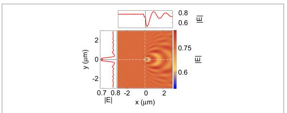
**Figure 7.** |E|-field map at the metal–prism interface. A cross-section of the nanoparticle is shown with a black circle. The |E|-field fluctuations are shown along the x-axis (top figure) and y-axis (left figure) passing through the centre of the nanoparticle.
