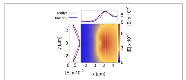
**Figure 9.** Plasmonic image (i.e. |E|-field) at z=950 nm from the metal–prism interface. The plasmonic image is plotted along the *x*-axis (top figure) and parallel to the *y*-axis at x=2.460  $\mu$ m (left figure), indicated with white dash lines, for both the analytical prediction (red line) and numerical calculations (blue line).
