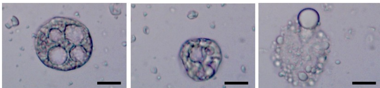
Figure 16. Light micrographs of cross-linked branched co-polymer-stabilised droplets performed at high concentration ( \Phi_{\text{oil}} 0.5 ). Note presence of droplet aggregation due to inter-droplet covalent cross-links. Scale bars represent 5 \mu\text{m} . Reproduced with permission from ref. 3.
