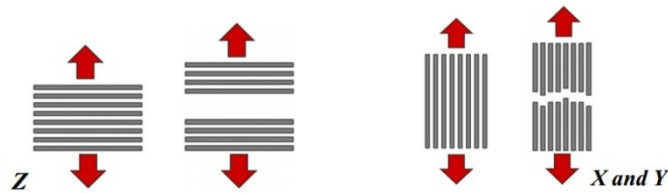
Figure 2.17. Schematic diagram illustrating differences in mechanical properties through different axes of the SLS part.
