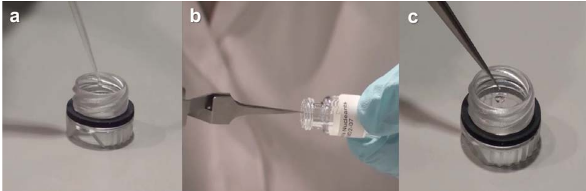
Figure 10: Technique utilized to add nucleant grains to crystallization drops. (a) crystallization droplet is dispensed, (b) vial containing nucleant is tipped slightly to dislodge a few grains and a single grain is picked up using fine tip forceps (c) addition of this single grain to a trial.
