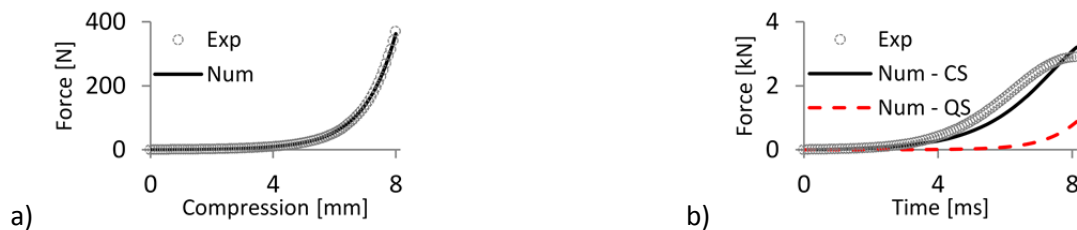
Fig. 2. a) Experimental and numerical results for the quasi-static test. The good match indicates that the derived material formulation is adequate ( n = 1 , C_0 = 25.6 kPa, C_1 = 13.6 ). b) Comparison between experimental and numerical results for a drop test of a velocity at impact of 1.3 m/s. The numerical results based on the quasi-static formulation (QS) do not predict the experimental output. Using the power law (CS) for strain-rate dependency ( C_p = 0.95 , C_D = 1.1 s -1 ), the FE model is able to simulate closer the result of the drop test.
