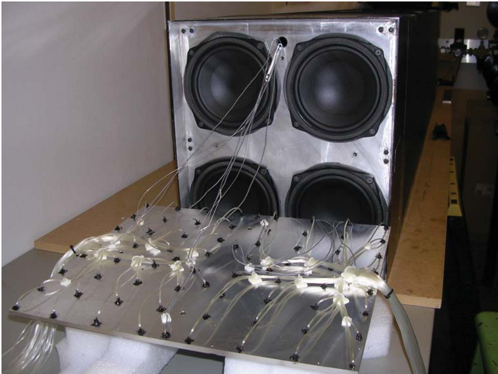
Figure F.3: Synthetic jet actuator set-up.
