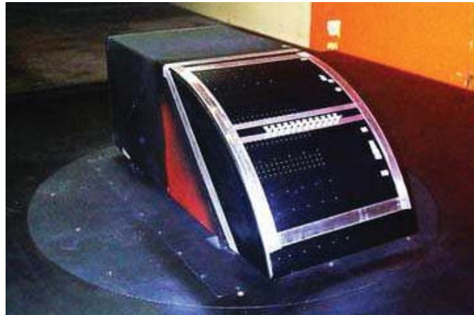
Figure 2.15: Picture of the rear of the model equipped with a set of VGs attached on a motorized rotating axis (Aider et al. , 2010).
