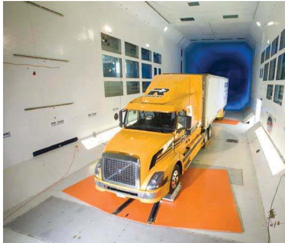
Figure 2.17: Volvo VN 660 and 28-ft trailer in the NRC 9 m \times 9 m wind tunnel (Leuschen & Cooper, 2006).
