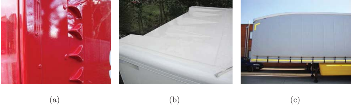
Figure 2.21: Aerodynamic devices applied to commercial vehicles: (a) vortex generators, (b) rear air diffuser and (c) roof line on both straight frame and double-deck that cants at the front (Montracon, 2013).
