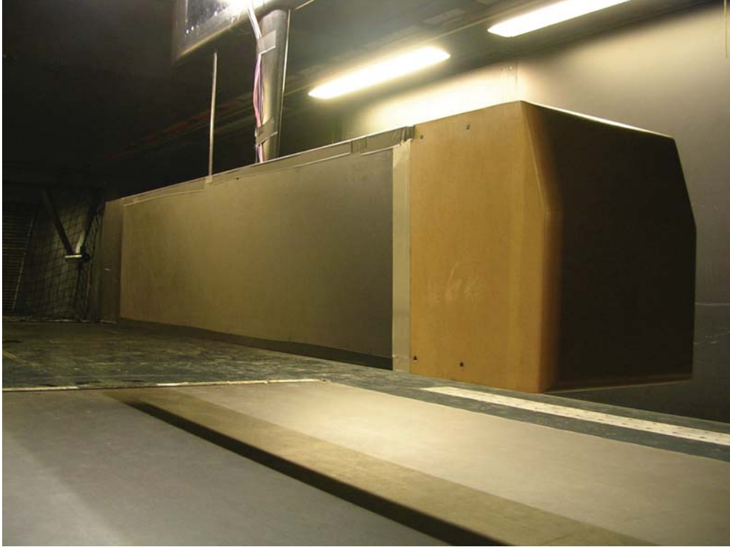
Figure F.5: Wind tunnel installation with model with square cab.
