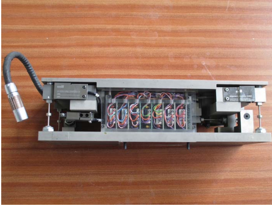
Figure 3.9: 6-axis internal balance used during the investigation.
