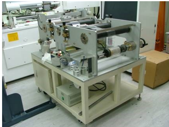
Figure 20: A “roll-to-roll” printing press equipped with a PDMS roller to imprints a pattern at high speeds onto a substrate. Fabricated by Industrial Technology Research Institute, Korea.
