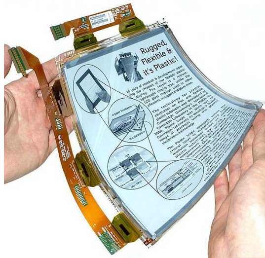
Figure 1: Photograph of a flexible electrophoretic display manufactured using OFETs by Plastic Logic.
