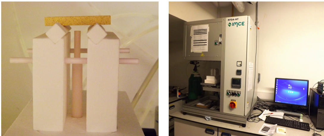
Figure 17 : A - Sample bar mounted on alumina hearth furniture at node points to ensure minimum damping of resonance. Ceramic striker tube centrally oriented beneath. B - Sample mount illustrated in A sits on elevator hearth which is raised into the furnace. Argon gas cylinder in background, used for inert gas atmosphere inside furnace.
