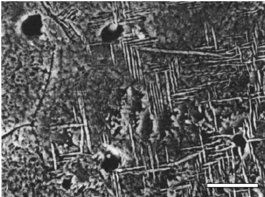
Figure 4 : Large random precipitates are often associated with lattice discontinuities such as pores. Image reproduced, with permission, from Hughan and Hannink 37 . Scalebar is 5 \mu\text{m} .
