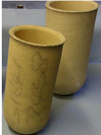
Figure 2 : Commercial Mg-PSZ refractory crucibles used for VIM of Ni-Co alloys.
