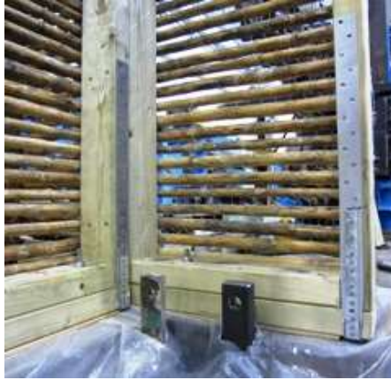
Figure 4. Detail of steel straps at the specimen ends
