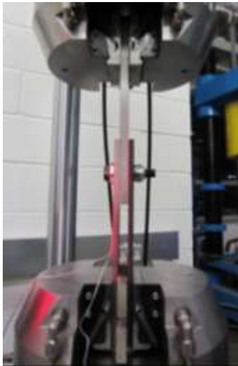
(b) Configuration Type B (double shear): general view (left) and test arrangement (right)
