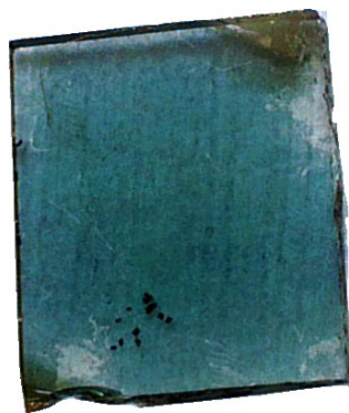
Figure 1 A picture of a 50 nm thick Au nanodisc arrays plasmonic substrate. The material is made up of gold, but does not reflect gold colour at all.
