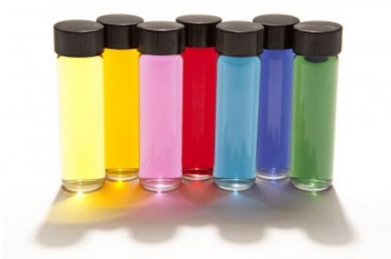
Figure 2-6 Solutions containing gold or silver nanoparticles of different nanoparticle sizes. From left to right: 80 nm Ag sphere, 20 nm Ag sphere, 40 nm Au sphere, 12 nm Au sphere, 200 nm Ag sphere, 120 nm Ag nanoplates, and 60 nm Ag nanoplates.. (Reprinted with copyright permission from nanoComposix.com.)
