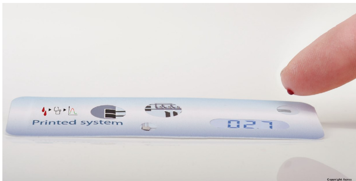
Figure 3-1 An illustration of an all printed disposable biosensor being developed by Acreo 121 . (Reprinted from ref 121 with permission from Royal Society of Chemistry.)
