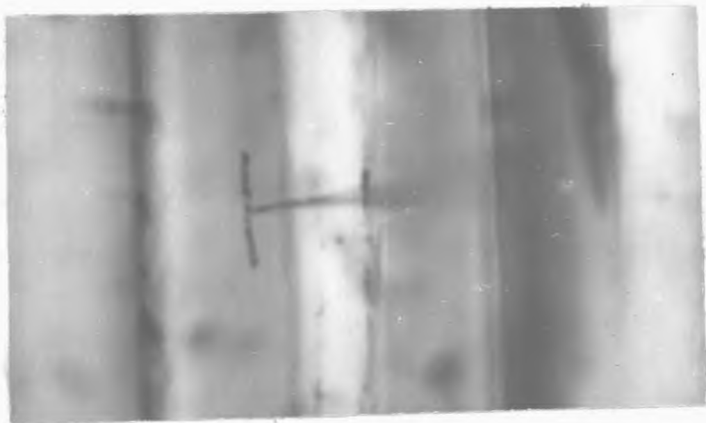
Fig. 27 - RIS Scots pine showing 'T-branch' formed by C. globosum in 6 weeks - 787 X
