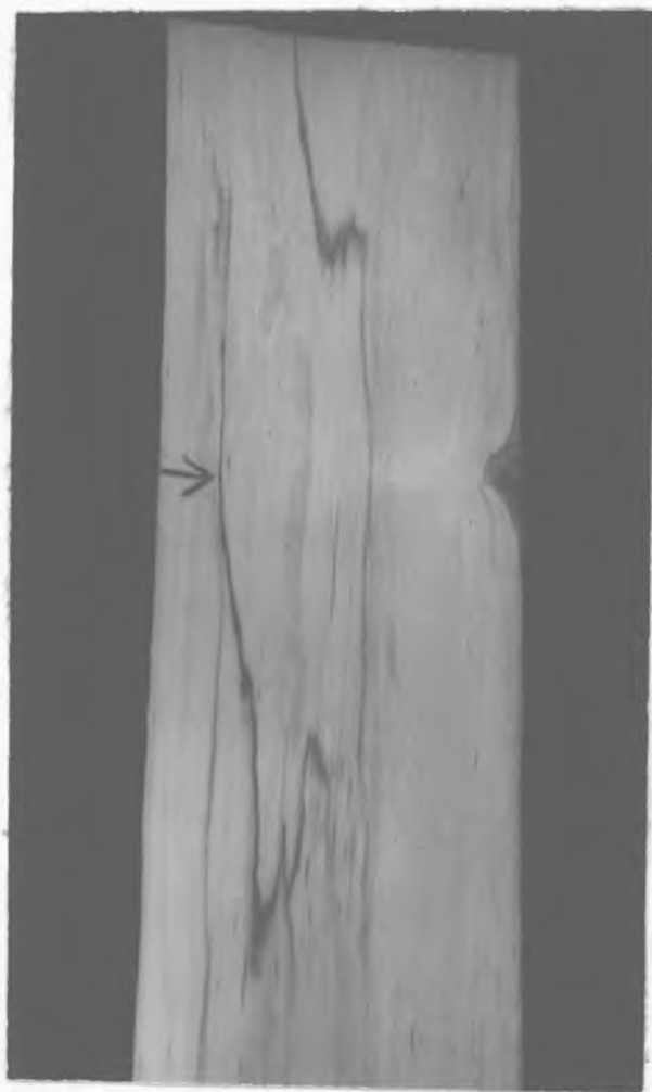
Fig. 2A - Birch post cut vertically to show discolouration and zonation by fungi inside the post. Arrow indicates the direction of sampling
