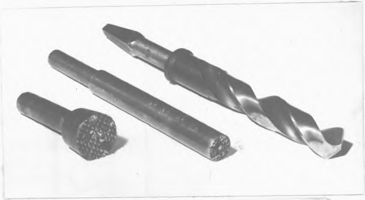
Fig. 1B - From left to right, (a) Surface grinder (b) Calibrated grinder bit for sampling base of hole, (c) Calibrated twist drill for boring hole.
