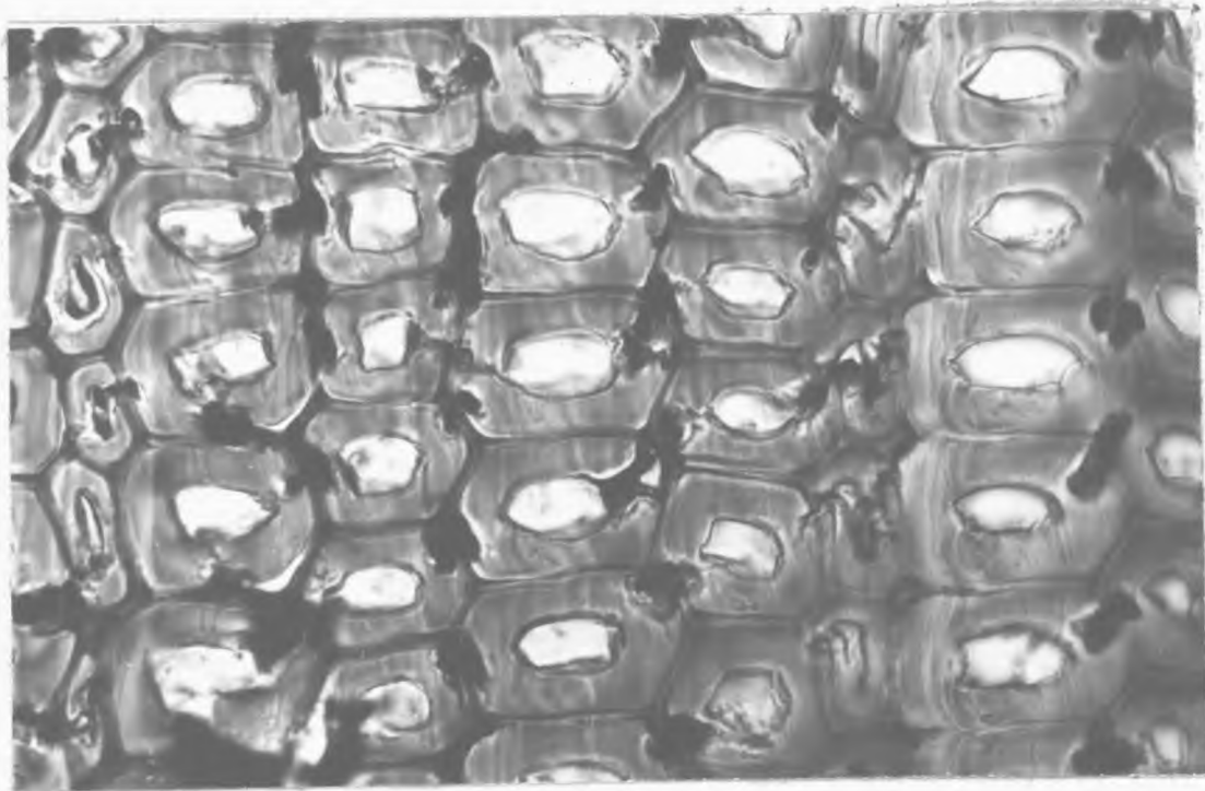
Fig. 29A - TS Scots pine showing colonization by C. globosum in the middle lamella and primary wall region, and forming cavities opposite to each other in the adjacent tracheid walls - 6 weeks - 320 X
