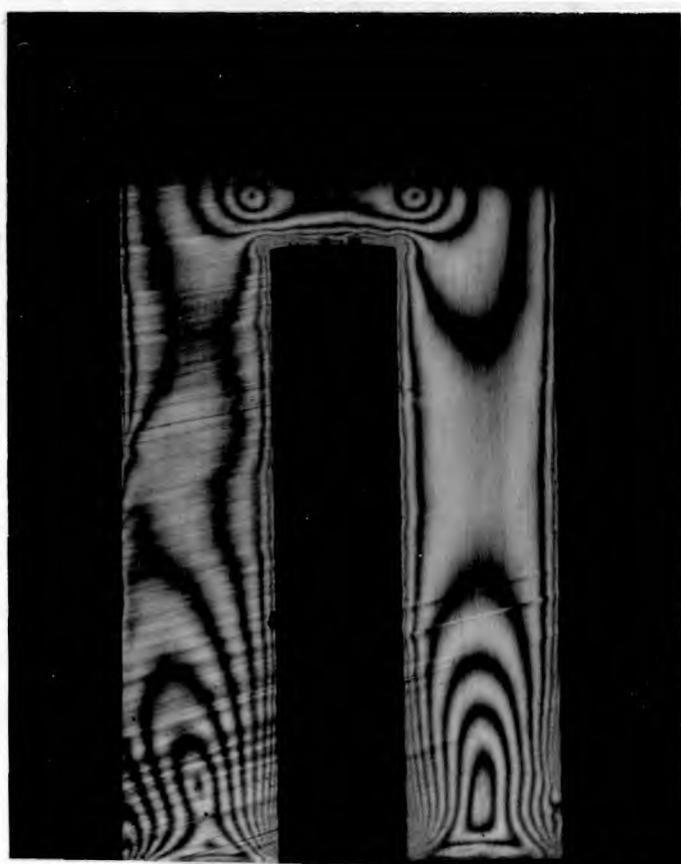
FIG.6.3e: TYPICAL ISOCHROMATICS FROM SLICE II FOR DISCONTINUOUS ROD ( m=4.5, \delta=\frac{1}{2} ). NOTE POSITION OF ISOTROPIC POINTS.
