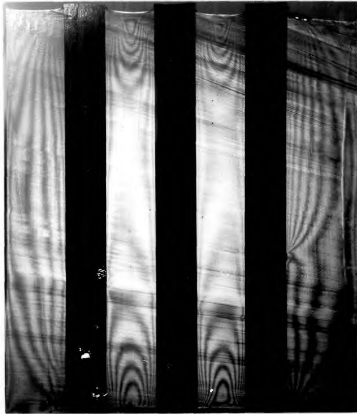
FIG6.3c: TYPICAL ISOCHROMATICS FROM SLICE II FOR CONTINUOUS RODS ( m=4.5, \delta=0 ).
