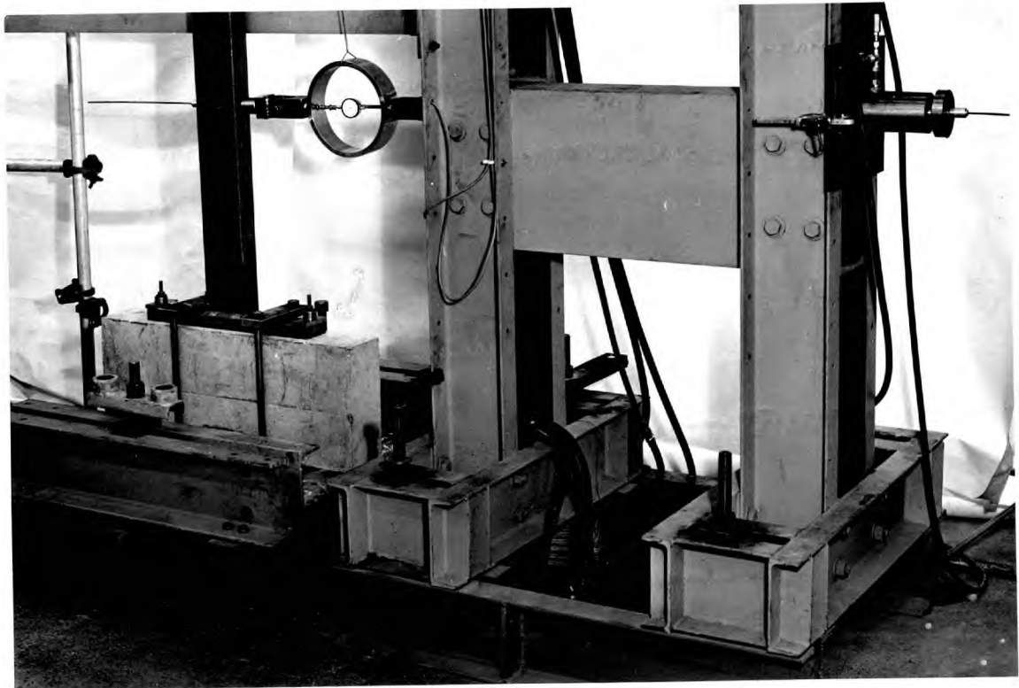
Calibration of Force-Moment Transducer
