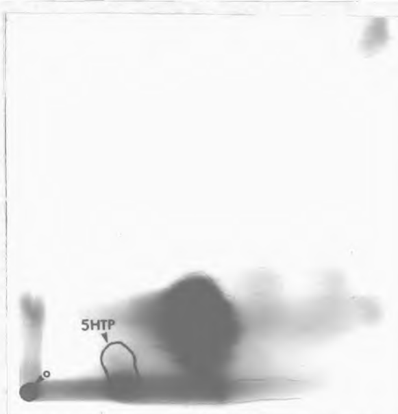
Fig. 14 Expt. 16 (Control) Radioautogram of two-way ascending paper chromatogram of extract from the incubation of BOILED tumour slices with DL-tryptophan- 3\text{-C}^{14} . Note there is little radioactivity in the area of 5HTP.
