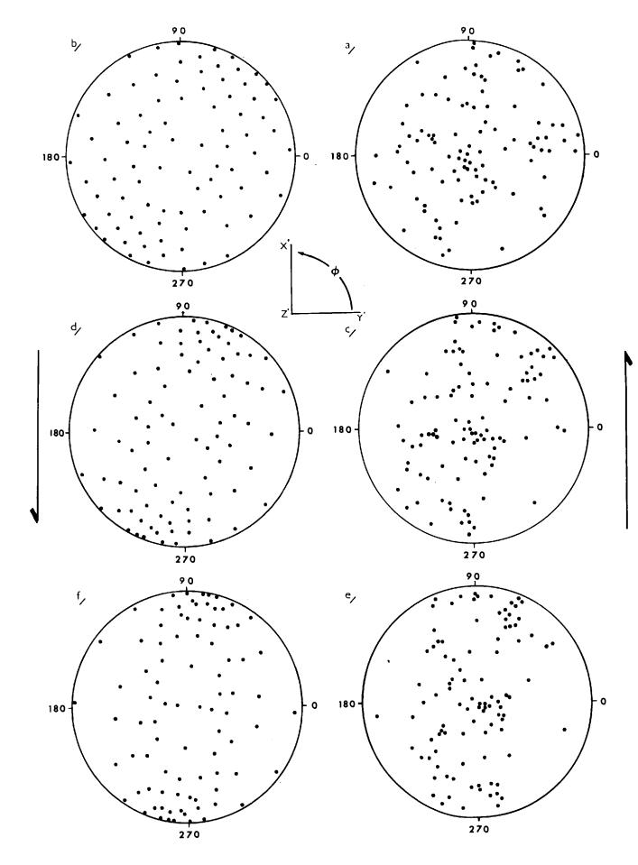
Figure 51 Stereographic projections showing the changes in the initially random and regular distributions of plunges of particle major axes (figures 49a, b) during pure shear. The axial ratios of the strain ellipses for each diagram are
