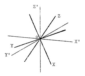
Figure 17 The two systems of rectangular coordinate axes used in the theoretical analysis.
