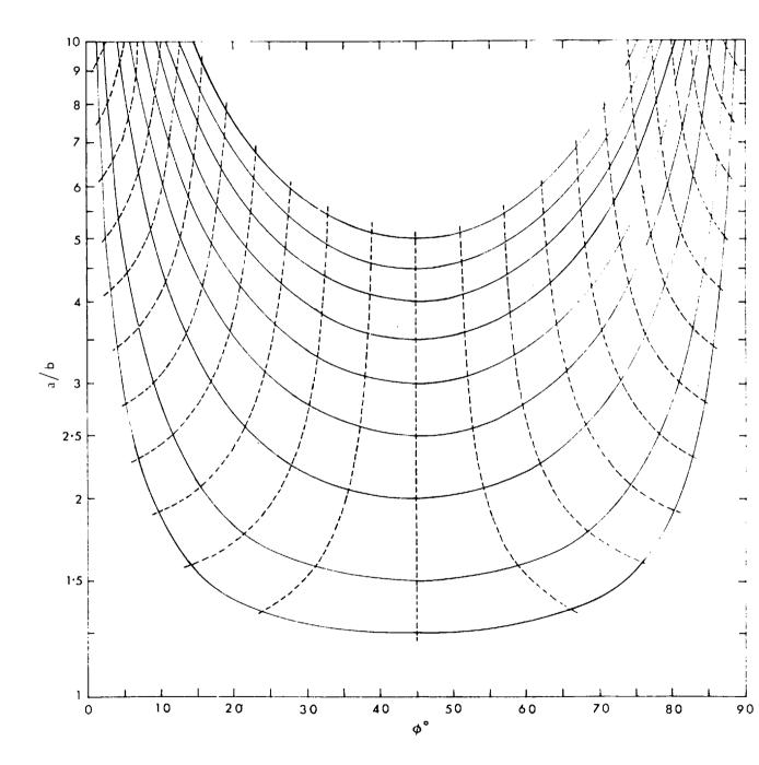
The results obtained from the computer were plotted graphically as in figure 33, which shows the changes, with deformation, of the shape and orientation of ellipses of any axial ratio for R = 1. The solid curves in this figure are the deformation paths followed by a particular ellipse while being strained. The dashed curves are contours of natural strain with a contour interval of  $\overline{\epsilon} = 0.1$ . Both sets of curves are symmetrical about  $\varphi = 45^{\circ}$ .
