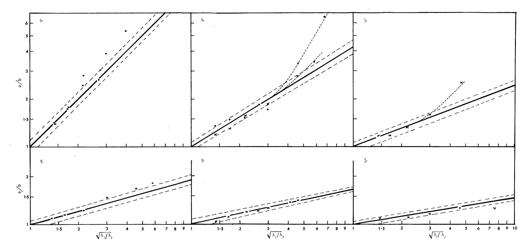
is good agreement between the theory and experimental results until the particle axial ratio reaches a value of about 2 : 1. However, beyond this point, the particles deform more rapidly than expected.
