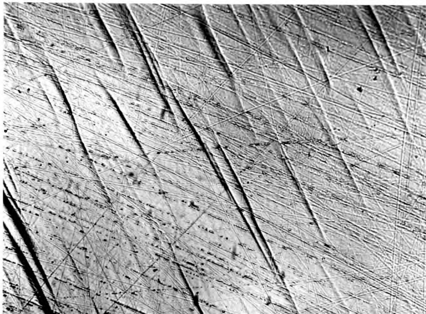
Fig. 4.12 (b) The slip lines after 10% strain; specimen mechanically polished after 5% strain and restrained. Mag x 540
