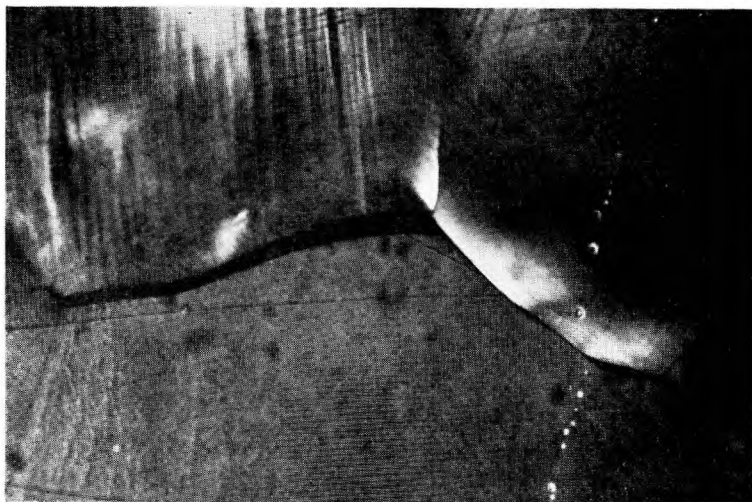
FIGURE 17.—Fine straight slip-lines observed after 2% compressive strain at 150°C ( \times 360 ).
