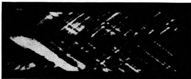
FIGURE 10.—Stress birefringence on Type D crystal compressed by 6% at 433°C ( \times 18 ).
