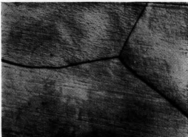
FIGURE 15.—Cracking of a grain-boundary triple point accompanying yielding at 120^{\circ}\text{C} ( \times 360 ).
