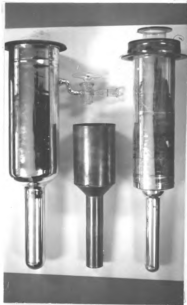
Plate 2. Showing the disassembled parts of the helium dewar.
