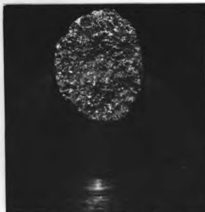
(e) 2.2:1, Cu:Mg alloy. Aged for 10 days. Tested at 295°K X6
