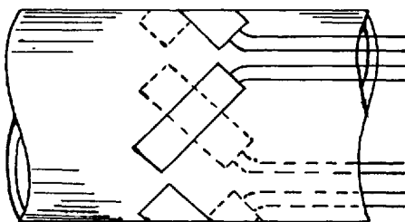
Fig.6.4 Arrangement of strain gauges on the shaft.
