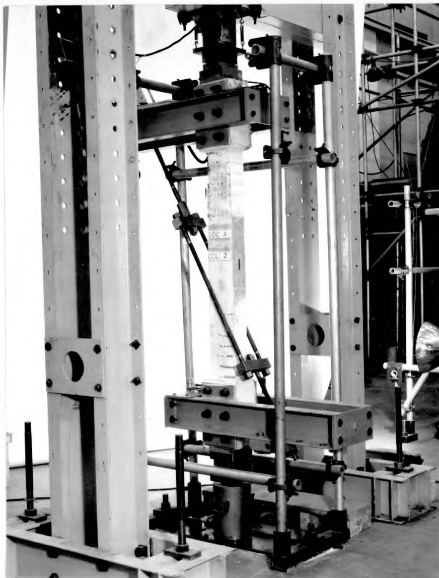
Plate 4.1 Test apparatus for columns under heavy axial load
