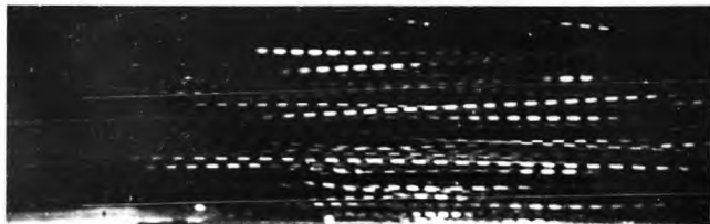
\theta = 150^\circ Centreline Q = 4.2 \times 10^{-3} \text{ m}^3/\text{sec} turbulent flow Chopper II
