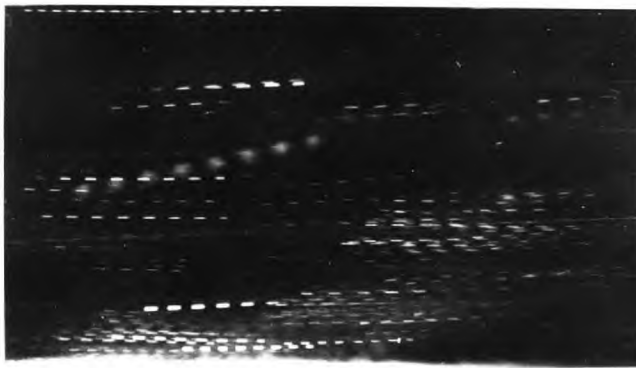
\theta = 30^\circ 15 cm from o/s Q = 0.2 \times 10^{-3} \text{ m}^3/\text{sec.} laminar flow Chopper I
