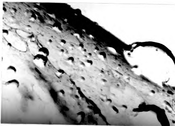
FIGURE 39. Electron microscope photograph of a replica taken of tin crystallites having a mean radius of several thousands Angstroms (x30,000).
