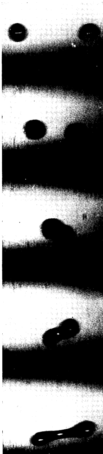
Figure 5. The coalescence of two drops of radius 120 \mu impacting at a relative velocity of 3 \text{ m sec}^{-1} . Photographs taken at 7,000 frames/sec.
