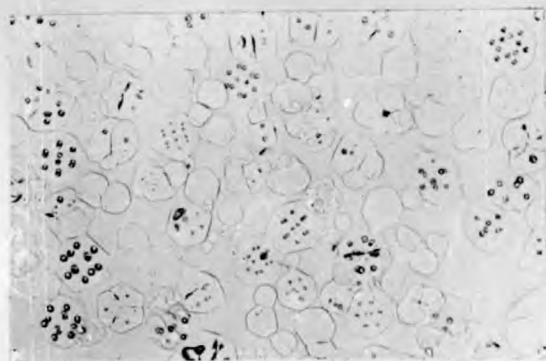
FIG . 7 - 14 . GROWTH OF HEXAMINE CRYSTALS . BATCH No 38 [ 100RPM , 40 °C , Full heat ]
