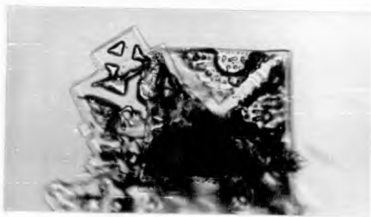
FIG. 9-2 PORTION OF CAVITITE CRYSTAL OF AMMONIUM CHLORIDE \times 70
