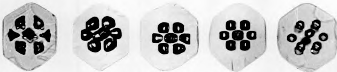
FIG. 7-41. CHANGE OF SHAPE OF INCLUSIONS IN HEXAMINE CRYSTALS WITH TIME. [x120]
