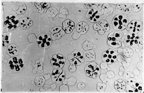
FIG.7-13. GROWTH OF HEXAMINE CRYSTALS. BATCH No. 37 [ 60 RPM , 40 °C , Full heat . ]
