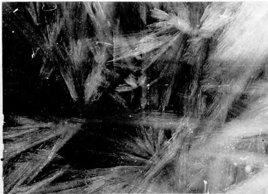
FIG. SII-1 . HEXAMINE HEPTAHYDRATE CRYSTALS GROWING IN SHALLOW DISH. [X2]
