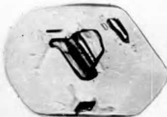
B. VARIOUS CRYSTALS GROWN FROM ETHANOL AND METHANOL SOLUTIONS, SHOWING SURFACE IRREGULARITIES OR DISTORTED SHAPES.
