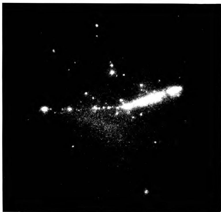
Fig.19(a). \pi \rightarrow \mu \rightarrow e decay in NaI(Tl) at 4:1 demagnification. ( \sim 25 \mu\text{A/lumen} photocathode.)
