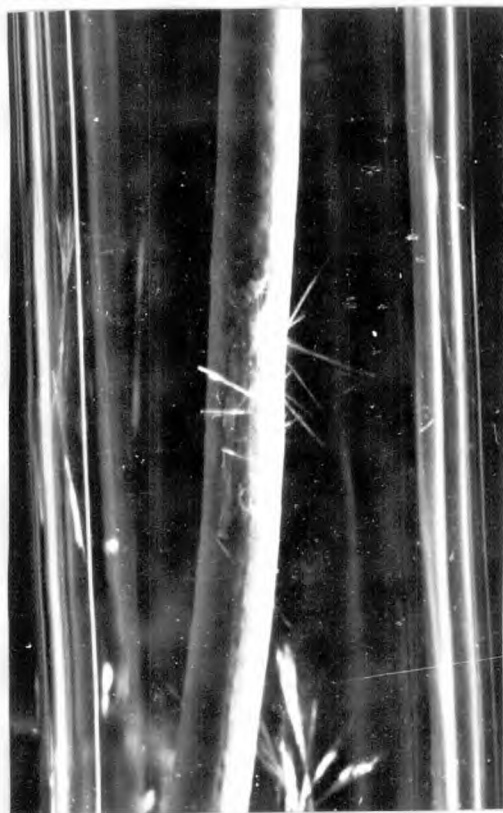
Painted galvanized iron wire with a scraped section (unstirred 4 hours)
