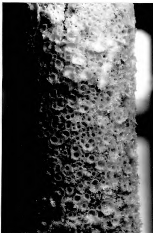
Run 377 Hemihydrate "rings" after 70 hours Magnification : 3x
