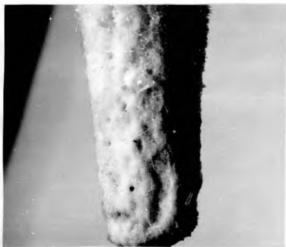
Run 595 Hemihydrate deposit at bottom of rod after 54 hours Magnification : 3x
