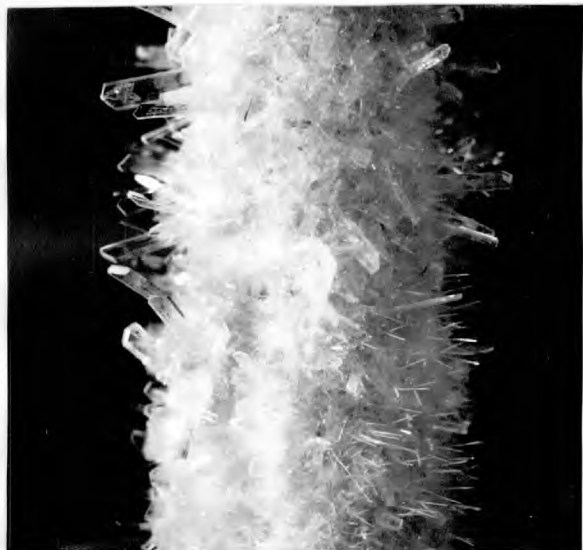
Run 595 Dihydrate (larger crystals) and hemihydrate deposit after 54 hours Magnification : 3x
