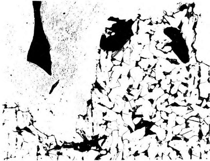
Fig. 9.2. Small chevron step edge.(x160).
