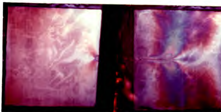
Fig. 7.9 Isochromatic pattern in the photoelastic coating on a specimen at 10°C and under a stress of 8 t.s.i. before (left side) and during (right side) brittle fracture propagation. The photoelastic coating is 10 inches square.
