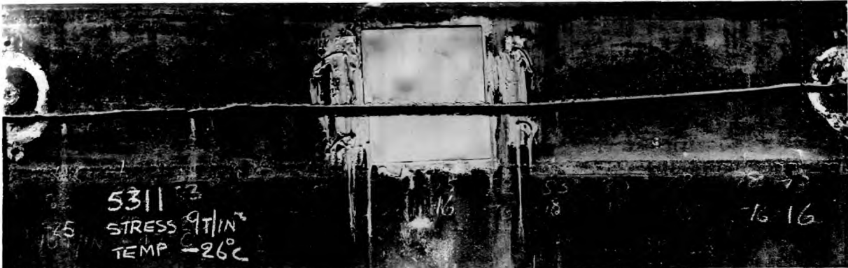
Fig. 7.38 6 foot wide specimen containing straight through fracture, 1/12 actual size.
