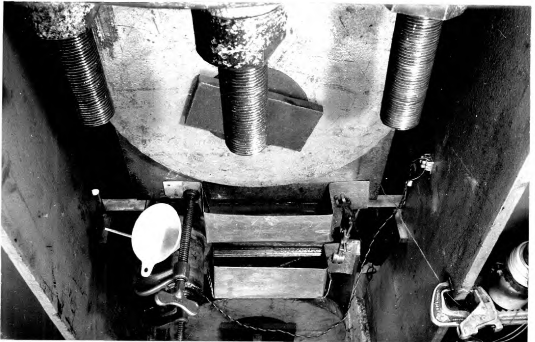
Fig. 6.1 Rear view of specimen mounted in 300 ton tensile rig, showing cooling trays and liquid nitrogen container/bullet catcher.
