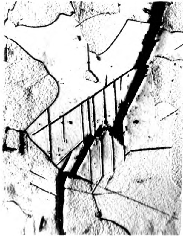
Fig.9.6. Twins crossed by a microcrack. (x800).
