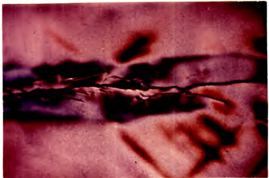
Fig. 7.28 The isochromatic pattern immediately behind a brittle crack. The area shown corresponds to fig. 7.27.
