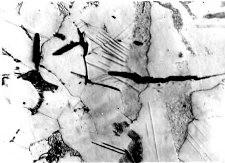
Fig.9.7 Intersecting twins associated with a microcrack.(x850).
