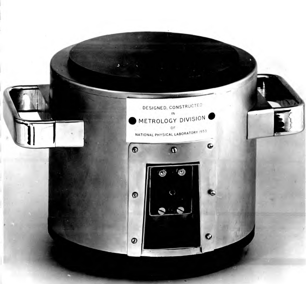
PLATE 2.2 150 tonf. electrical resistance strain gauge load cell used as a secondary load standard at the National Physical Laboratory
