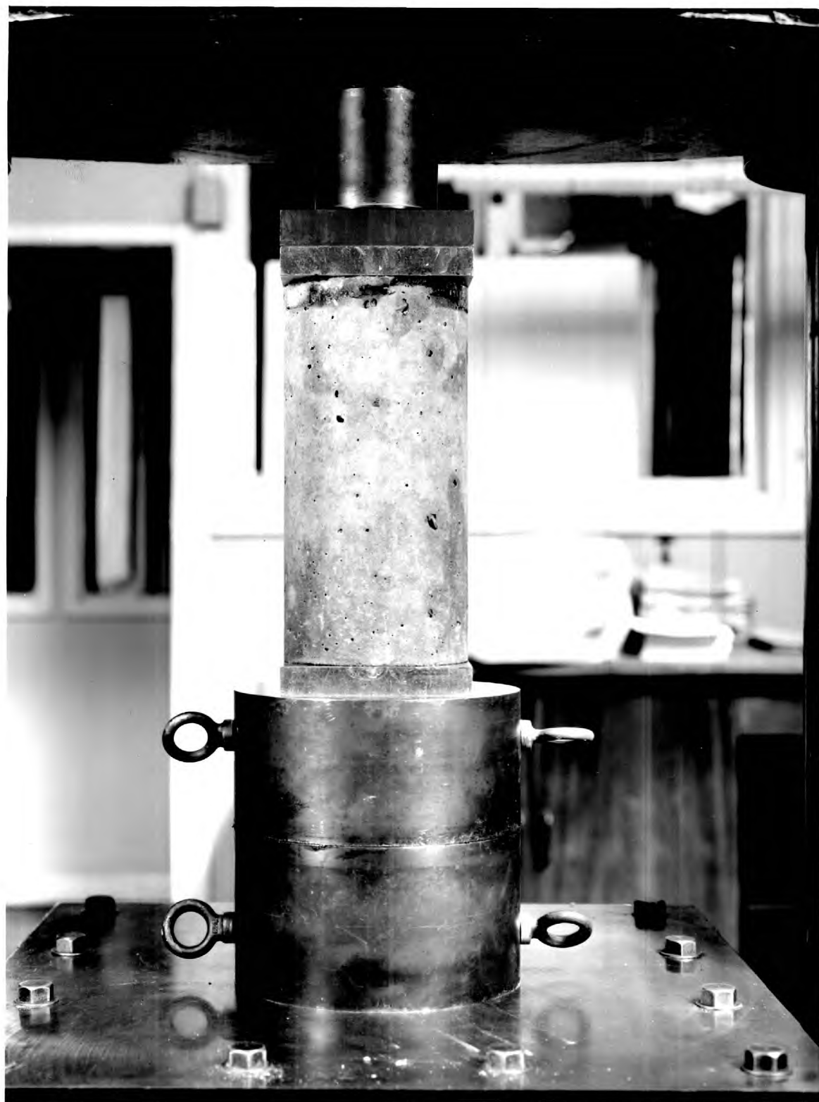
PLATE 9.1 Test assembly for loading concrete specimens under both ends pinned condition
