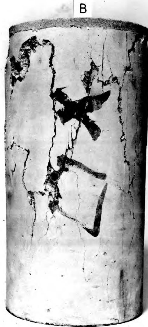
PLATE 9.3 Concrete cylinder loaded to failure with both ends effectively fixed
