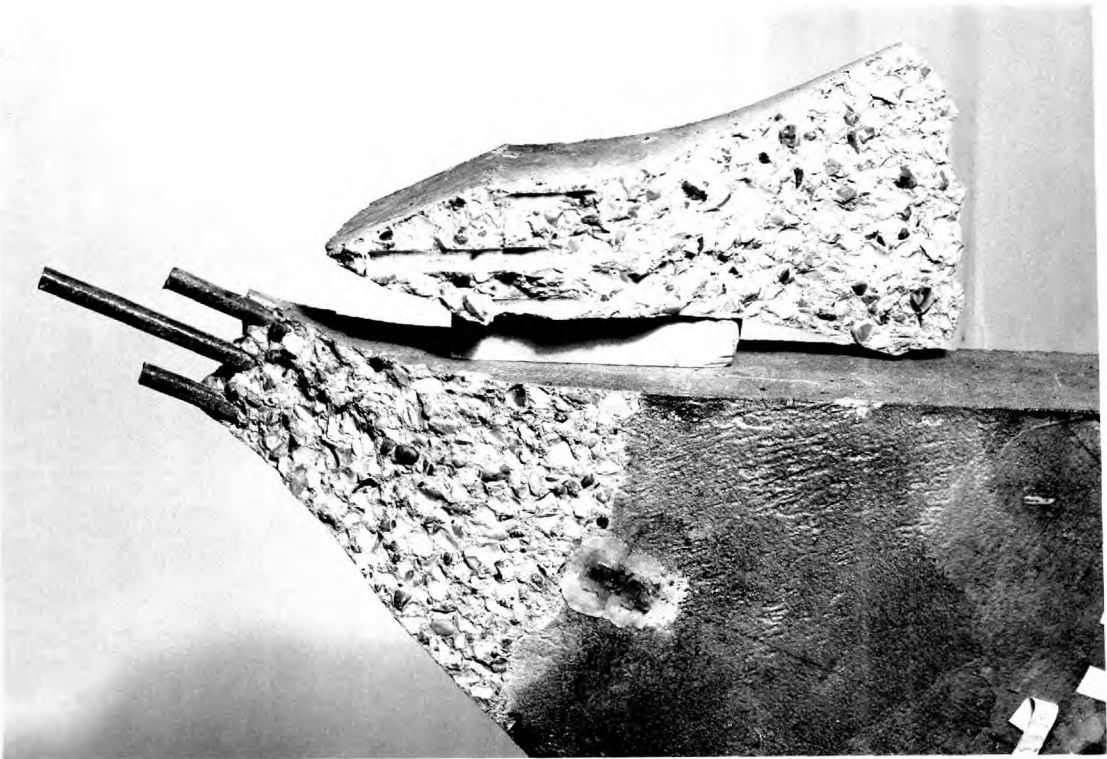
PLATE 18.2 Initial slab specimen at failure
