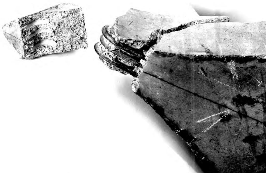
PLATE 18.4 Second slab specimen at failure
