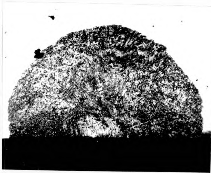
FIG.6(a) Photo - Micrograph showing an approximately hemispherical nodule of pearlite growing from the surface of the specimen. x 80
