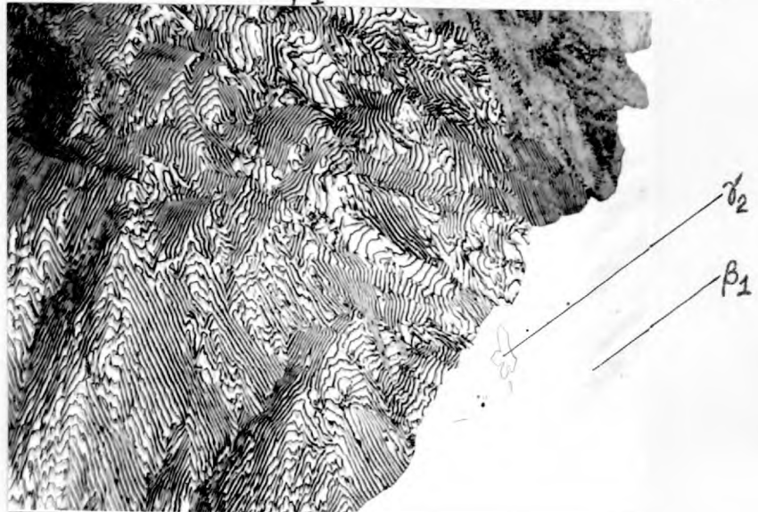
FIG.20 Precipitation of \delta_2 with the formation of \beta . The background is \beta_1 . Temp. 525°C. x 525
