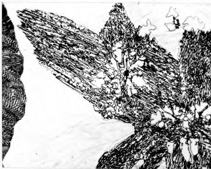
FIG.54 \alpha and \gamma_2 mixture from the decomposition of the \beta phase, resulting from the precipitated
