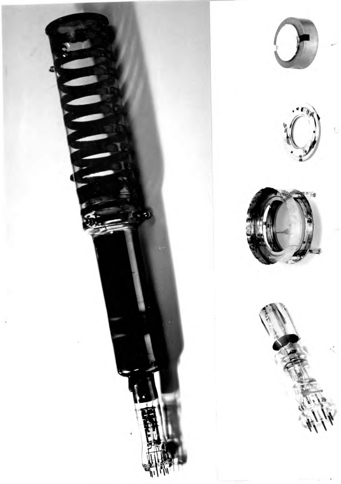
Fig. 7.2 Camera Tube and Internal Parts
