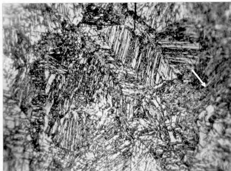
Fig.44: Martensite plates formed 5^{\circ}\text{C} below M_s under a stress of 53,000 \text{ lb/in}^2 .
