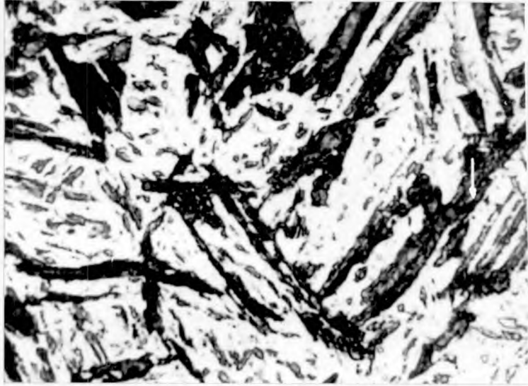
Fig.37: Martensite plates formed 5^{\circ}\text{C} below M_s under a stress of 8,000 \text{ lb/in}^2 . The direction of stressing is shown by white arrows. x 1200.
