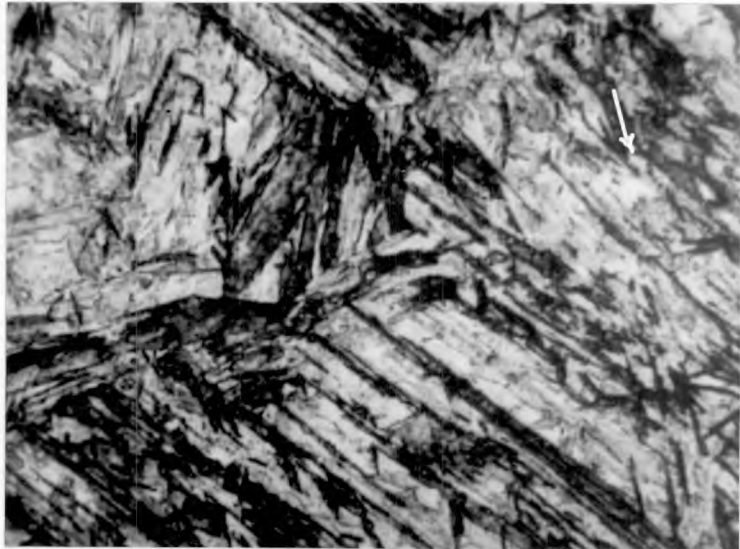
Fig.42: Martensite plates formed 5^{\circ}\text{C} below M_s under a stress of 35,000 \text{ lb/in}^2 .
