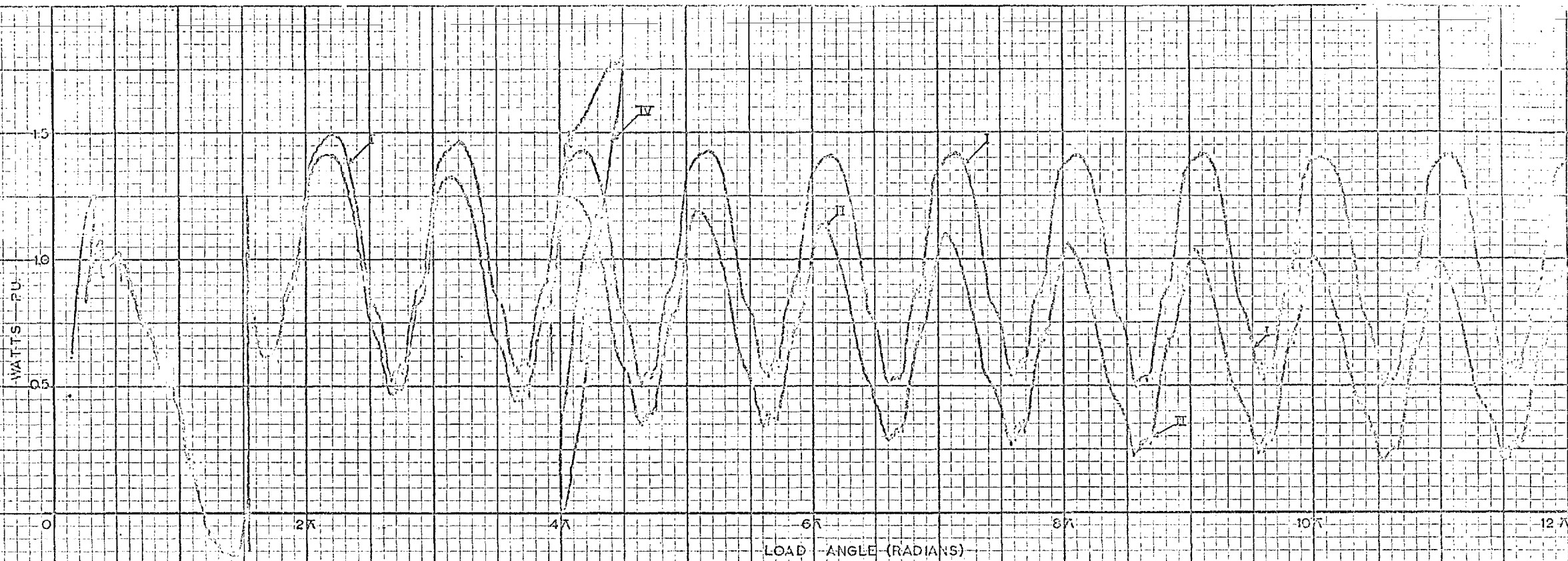
Fig. 6.13(c) Watts - Load angle (Governor: T_g = 4.0 sec., Droop = 4.0%)
