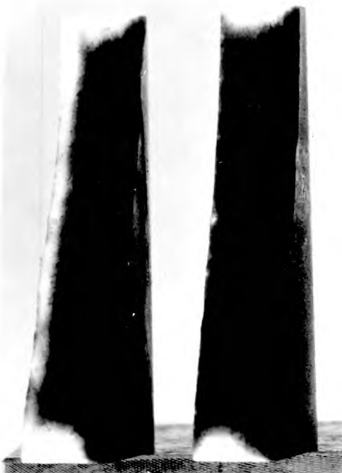
20a Dye impregnation of hot and cold zone wall sections parallel to tube axis (hot section on left)
