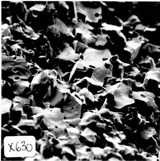
27a Scanning electron micrograph of hot zone tube interior (normal to tube axis)
