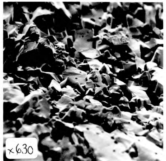
27b Scanning electron micrograph of cold zone tube interior (normal to tube axis)
