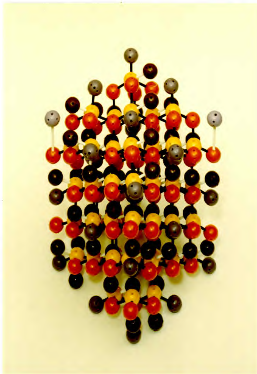
FIG. 10 Hypothetical structure of bornite showing atomic layers parallel to (111)_{rh} . (White unions should be ignored).
