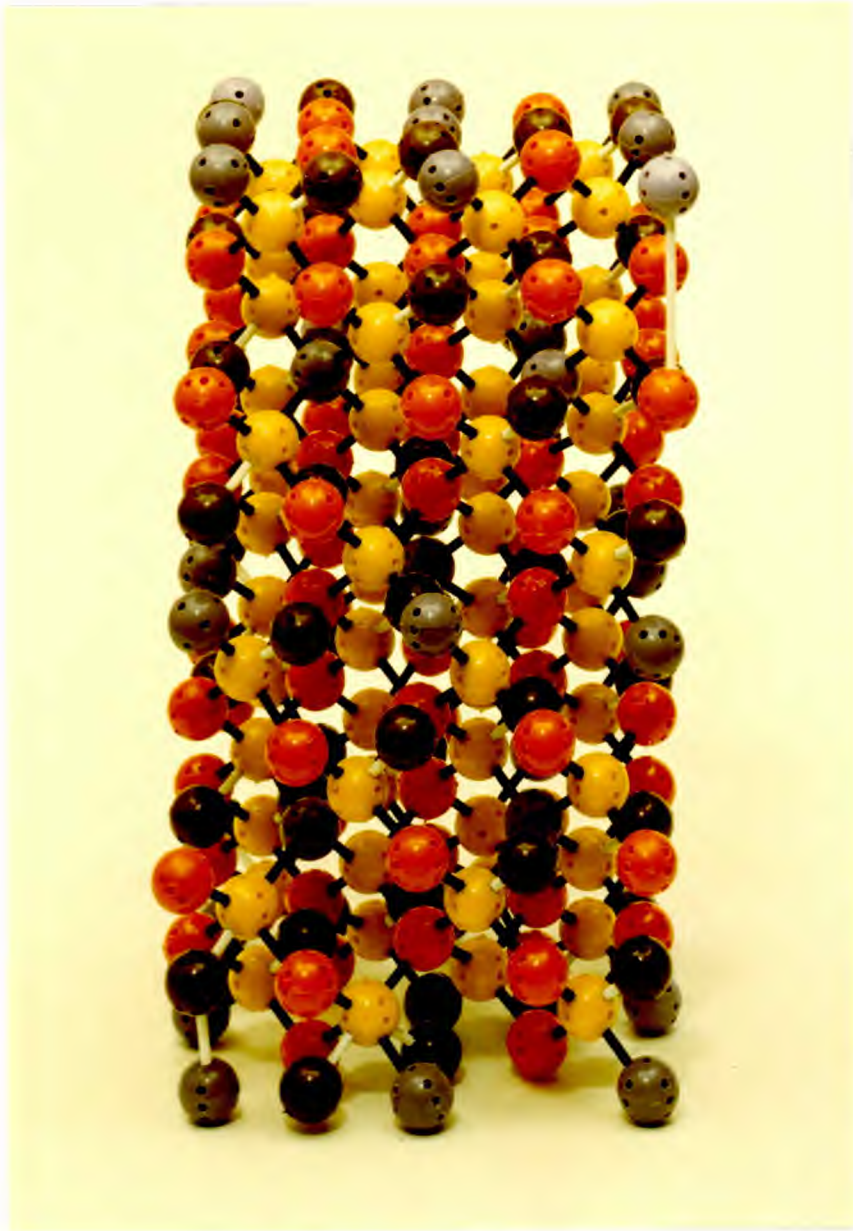
FIG. 9 Hypothetical crystal structure of the low temperature form of bornite. The \text{Cu}_7\text{FeS}_4 sphalerite-type skeleton is formed by sulphur atoms (yellow), iron atoms (blue) and copper atoms (orange). The interstitial, ionically bound copper atoms are shown in brown.
