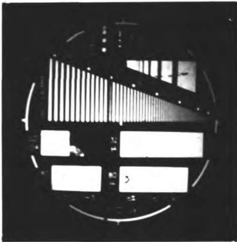
(c) Image on a phosphor in the target plane (Baum pattern ~ 8mm. diameter M \sim 1 ) EHT = 7.5KV.
